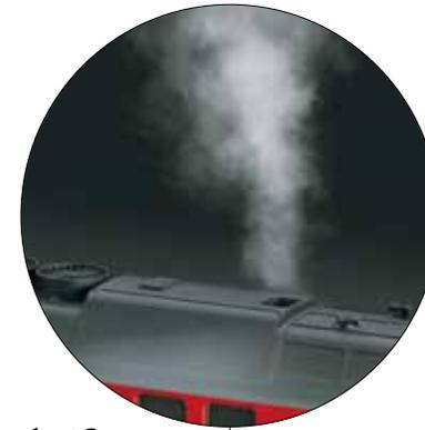
*Cold water-based smoke unit that can be controlled digitally in 3 steps*
