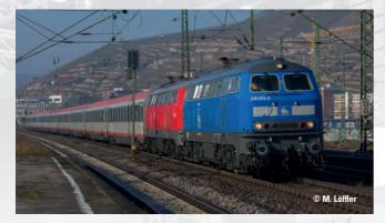
**Prototype**: Pressnitz Valley Railroad, Inc. (PRESS) class 218 diesel hydraulic locomotive in a traffic blue paint scheme. B-B wheel arrangement. The locomotive looks as it currently does in real life.
