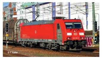
**Prototype**: Traxx 2 electric locomotive, type F 140 AC2 for the firm DB Schenker Rail Scandinavia A/S, a cooperative venture between DB Schenker Rail Germany, Inc. and the Swedish Green Cargo AB. The locomotive looks as it did in 2017/18. The area of use is Denmark and also into Germany.
