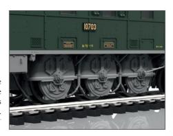
While the wheel centers on the right side are easy to recognize, the Buchli drive on the left side of the prototype is predominant on the model. The transmission of the torque to each of the individual axles is done through the link drive surrounded by sand pipes.
