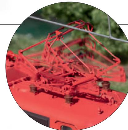
Pantographs can be raised and lowered digitally
