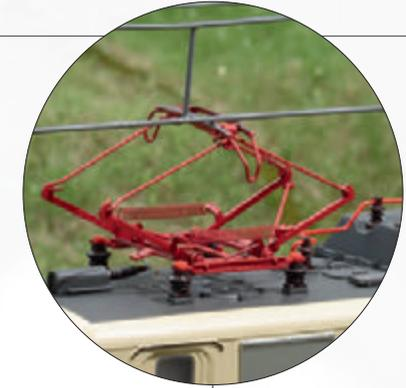
Newly designed type DBS 54 pantographs can be raised and lowered digitally
