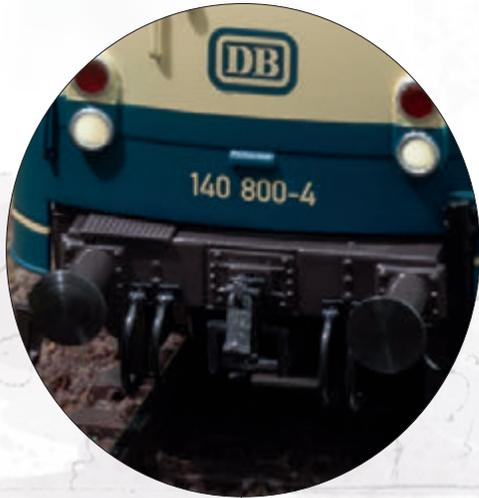
Buffer height adheres to the NEM and close couplers with a guide mechanism
